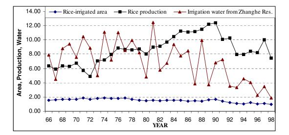
**Fig. 2** Annual rice-irrigated area (10<sup>5</sup>ha), rice production (10<sup>8</sup>kg) and irrigation water (10<sup>8</sup>cubic meters) from Zhanghe Reservoir (1966-1998)
